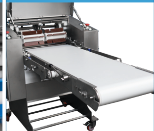
Long infeed conveyor = +546mm
