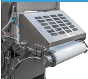
Short outfeed conveyor ≈ 607mm
